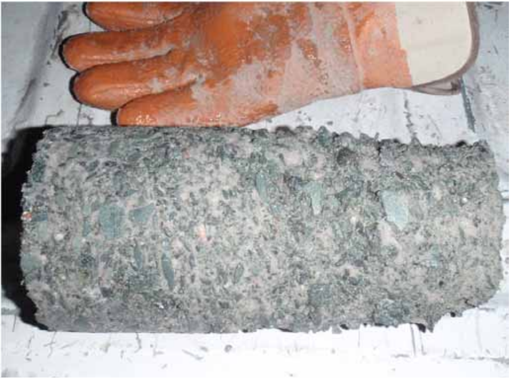
Photo 6: Drilled Core 19 (HB12-ND-CORE-DC19-QA-20120203). Core taken from ~0+42 downstream.
