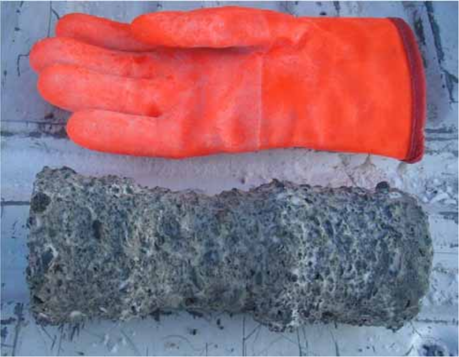
Photo 4: Drilled Core 17 (HB12-ND-CORE-DC17-QA-20120203). Core taken from ~1+00 US. Poor quality of core is due to dislodged gravel spinning/ drill spin.
